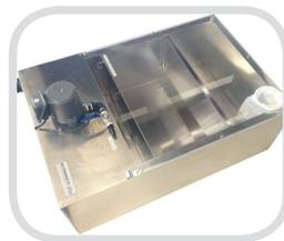
Compound re-cycling system complete with basic solids filtration. Fitted with single phase pump and under over baffle plates.
