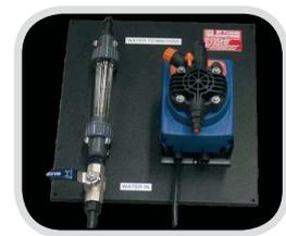
Compound & water dosing system. Incorporating adjustable water flow meter and chemical dosing pump allowing precise regulation of water and compound to the finishing process.
