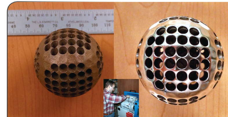
A three-step, hands-free, high-speed centrifugal iso-finishing process was used to reduce the surface roughness on this 3D-printed metal component from 356.24 micro-inches Ra (left) to 12.06 microinches Ra (right). (Images and profilometric data courtesy of Jack Clark, Surface Analytics.)
