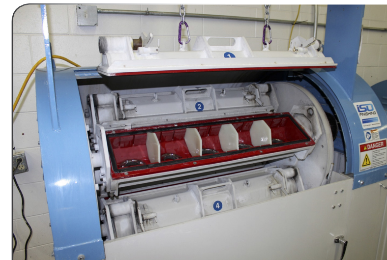
Centrifugal iso-finishing can produce very refined surface finishes on parts in abbreviated process cycle times. (Image courtesy of Cole Mathisen, MFI.)
